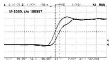
Upper trace is Channel 2. This is the input current viewed across a 50 Ohm termination. The lower trace is from the 6585 under test. The units under test were placed in a coaxial test fixture. Equal length cables were used from the fixture and the CT under test to the oscilloscope.
