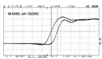
Delay is measured by placing the cursors on the zero crossings. The signal step is centered vertically on the zero axis. The delay is at the lower right corner of each figure ( $\Delta t =$ ).
