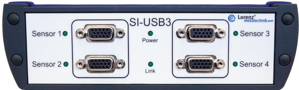
The four sensors are signed with Sensor 1 - 4. First the power supply must be connected. When a sensor is connected, the corresponding power LED is activated. Only when a PC/Laptop connection via the USB socket on the back exists, the Link-LED is activated. If the Link-LED is dark, check again the connection SI-USB3 to the PC/Laptop. Temperature measurements are possible at sensor connection 1 and/or sensor connection 4.
