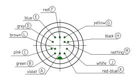
View: socket on soldering side
