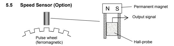
A hall sensor is located between the pulse wheel and the permanent magnet. If a tooth of the pulse wheel passes the energized hall sensor, the field intensity of the permanent magnet changes. By this, hall voltage occurs which is processed to a rectangular signal by the integrated evaluation electronics.
